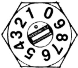
Increased opening may be necessary for lower temperatures. When adjusting counter clockwise rotation will increase flow clockwise rotation will decrease flow for your individual requirements. Adjust to the point where a
