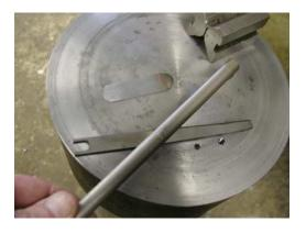
Remove Shim and test that the leg moves freely.
