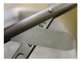
Place shim between leg and spindle on each side of pin.
