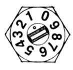
The adjustable feeder makes it adaptable to all climates and conditions. The new improved feeder will not move under vibration. The normal setting is for summer conditions with a No.10 oil.
