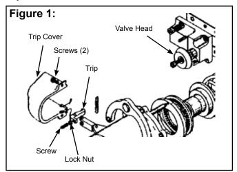
Remove the two screws to remove the trip cover, see Figure 1. The trip engages the valve head. There should be approximately 5/64" clearance between the outside diameter of the valve head and the notch of the trip when in the proper operating position. If adjustment is necessary, use a 5/64" (.078") diameter drill as a gauge.
